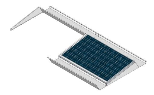
As all components are metal, frameworks modules and structure are equipotentially joined, making ground connection easier.
